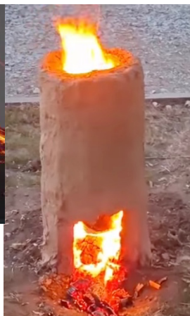
An Iron-Furnace made of clay.
